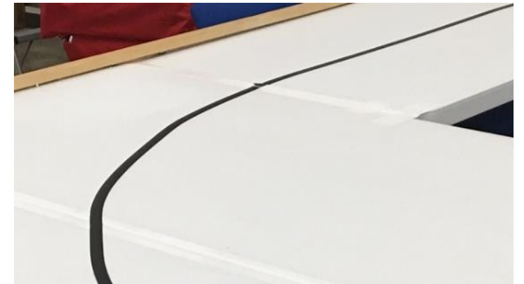
d) Finished connections with 2" tape and black line from electrical tape
